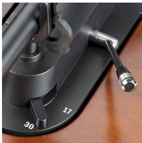
The small lever at the front of the tonearm board is typical for dual automatic turntables and is used to set the device to LPs or singles.
