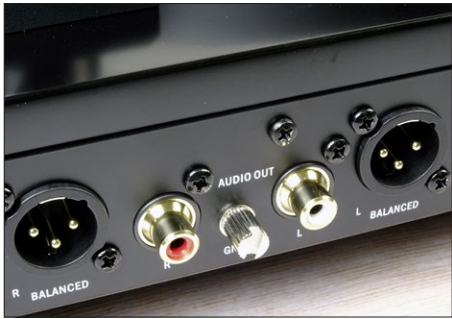
In addition to the RCA sockets, there are three-pin XLR contacts for the balanced connection.
