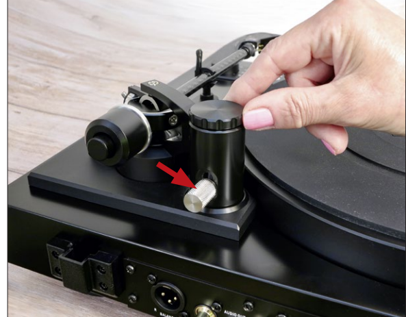
After loosening the retaining bolt (arrow), the arm base can be moved vertically via the screw.
