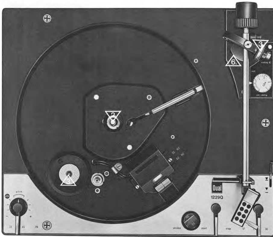
Fig. 30 Lubrication points above the chassis
