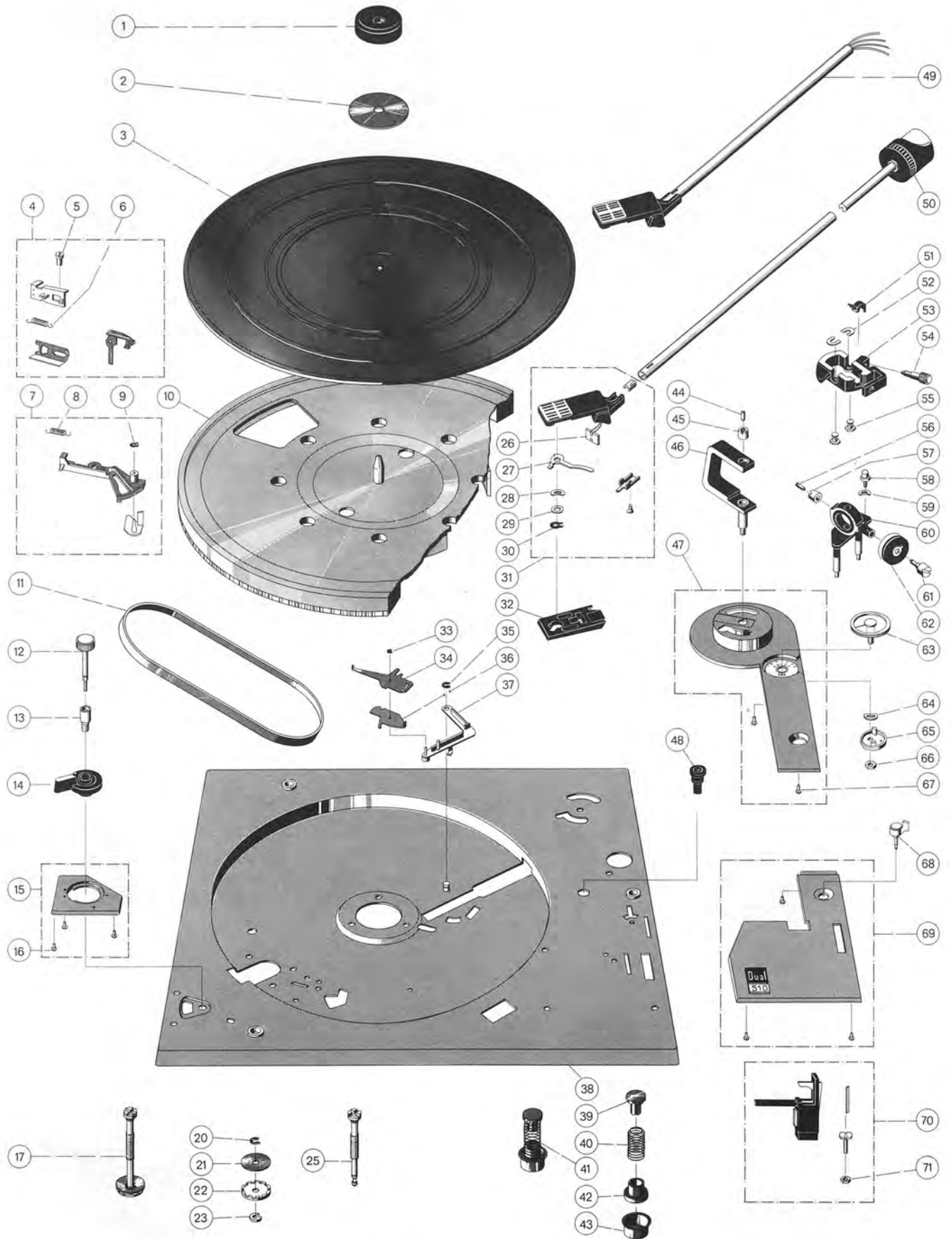
Fig. 19 Exploded view above chassis
