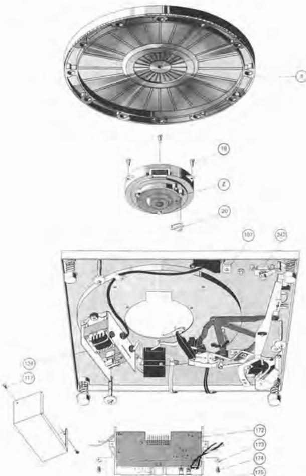
4. Pull off motor electronic system from motor (18) carefully.
