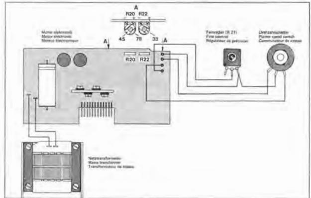
Fig. 7 Power Supply Board (component side)
