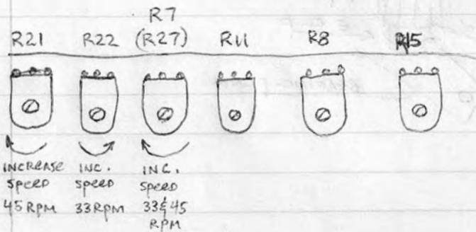
LIGHTED STROBE WORKS FOR 33 1/3 RPM ONLY, READ 45 RPM ON CENTER DISC
